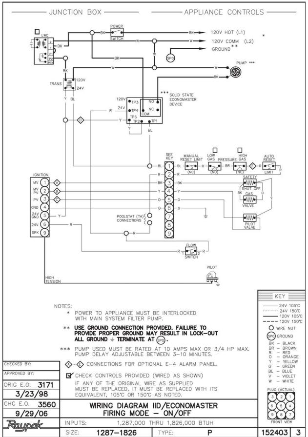
WIRING DIAGRAM MODELS 2100-2500
